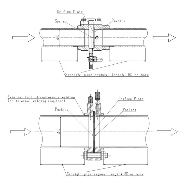
% After completing the piping work, be sure to check that there is no misalignm ent of the internal orifice plate.
